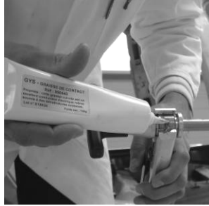
❷ Add copper grease on the inside of the clamp and on the axis of the tool.
